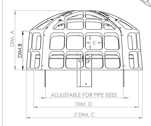
**PART INFORMATION** PART NO. RSP-36 DIM. A 21-1/4" 14-3/8" DIM. B DIM. C 40-7/8" 37-1/2" DIM. D 4-1/2" X 5" MIN. DIM E VARIES 6-1/2" x 5-7/8" MAX. 34" MAX PIPE OD. 23" MIN. PIPE ID. MOUNTING KIT ANGLE 1-1/4"X1-1/4"X3/16" HDPE ANCHOR PLATE 12"X4"X1/4"
